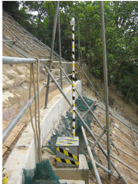
Figure 2 – Wireless local datalogger and antenna, at top of borehole
